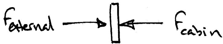
$$\begin{aligned} F_{cabin} - F_{external} &= (P_{cabin} \times A) - (P_{external} \times A) \\ &= (1 \times 10^5 \times 2) - (0.4 \times 10^5 \times 2) \\ &= 2 \times 10^5 - 0.8 \times 10^5 \\ &\leq \underline{1.2 \times 10^5 \text{ N}} \end{aligned}$$
