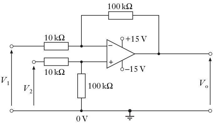
When  $V_o = 0\cdot60\text{ V}$  and  $V_1 = 2\cdot70\text{ V}$ , what is the value of  $V_2$ ?
