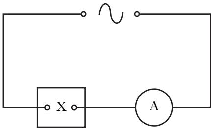
As the frequency of the a.c. supply is steadily increased, the ammeter reading also increases.
