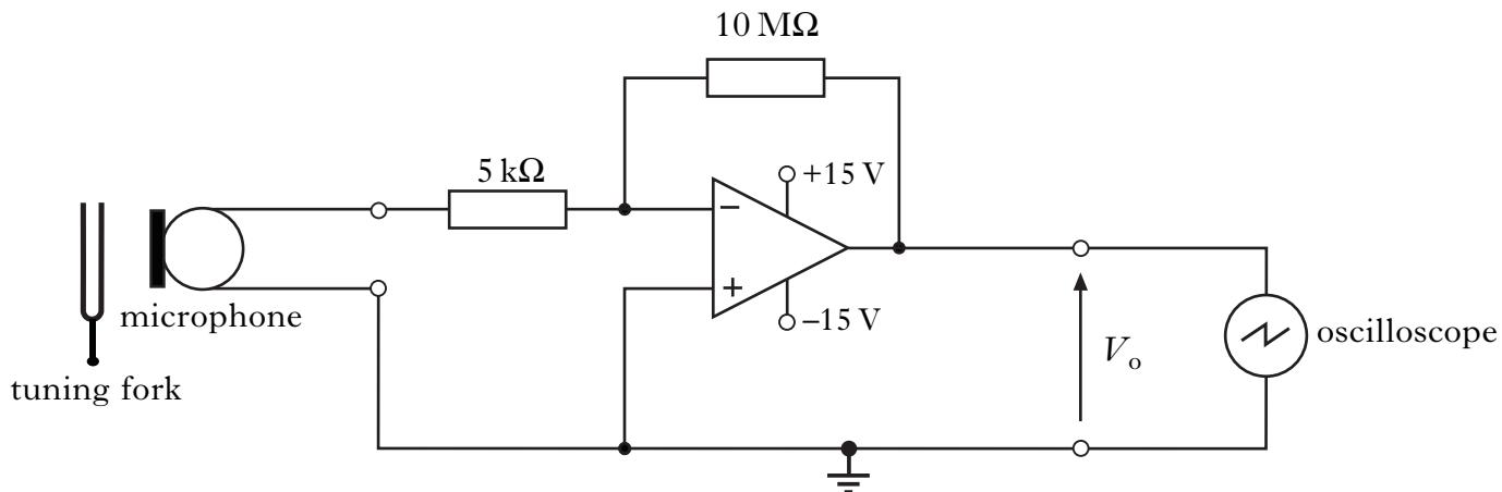
The settings of the oscilloscope are adjusted to show a trace of the amplified signal.
