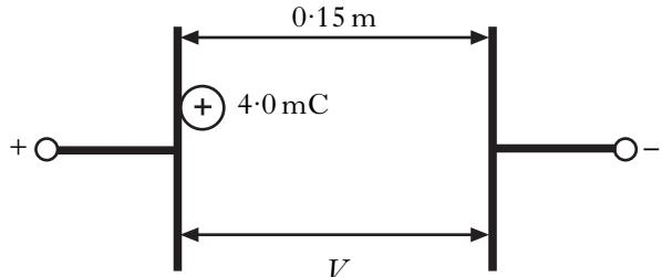
The kinetic energy of the charge just before it hits the negative plate is 8·0 J.
