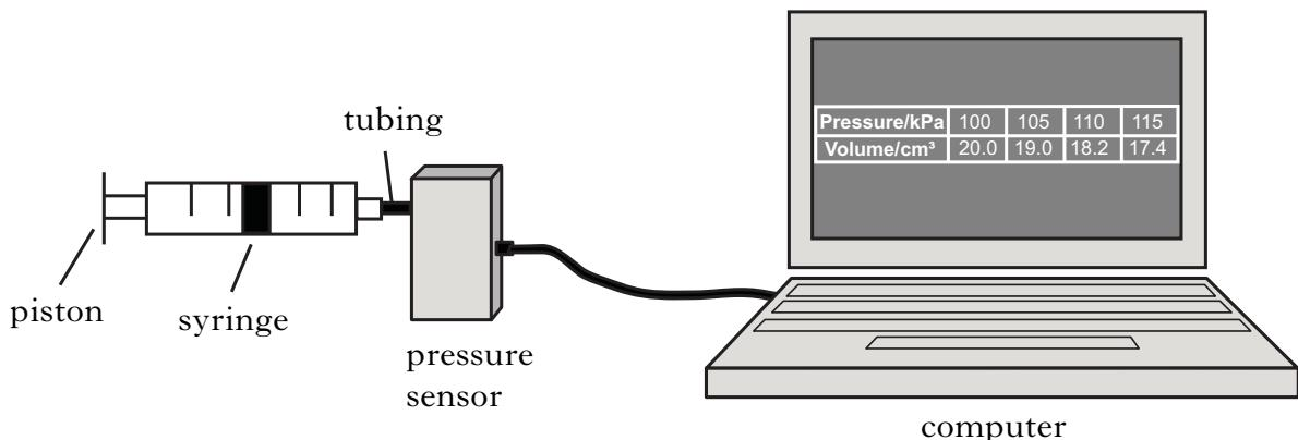
The pressure of the gas is recorded using a pressure sensor connected to a computer. The volume of the gas is also recorded. The student pushes the piston to alter the volume and a series of readings is taken.
