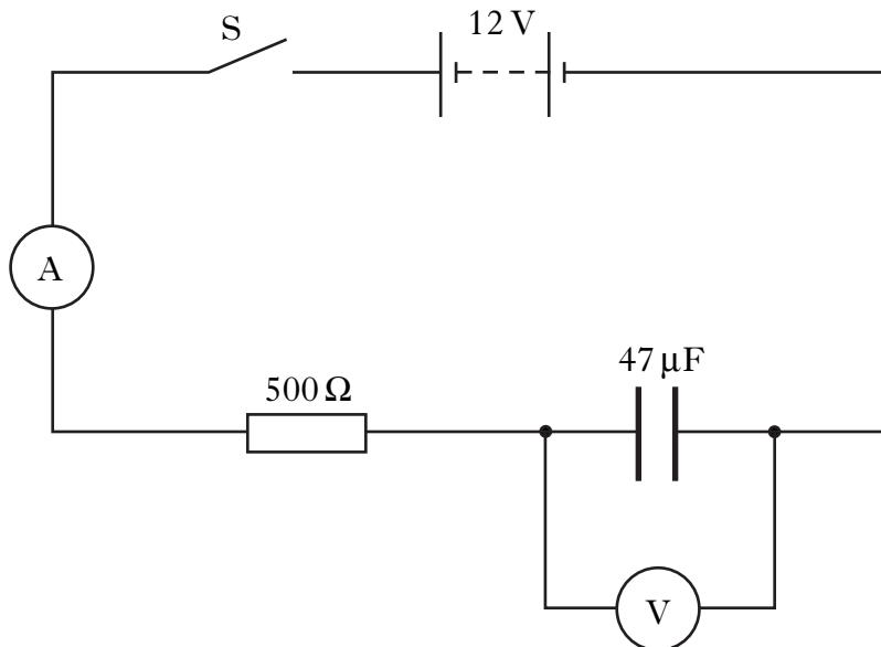
The capacitor is initially uncharged. Switch S is then closed and the capacitor starts to charge.
