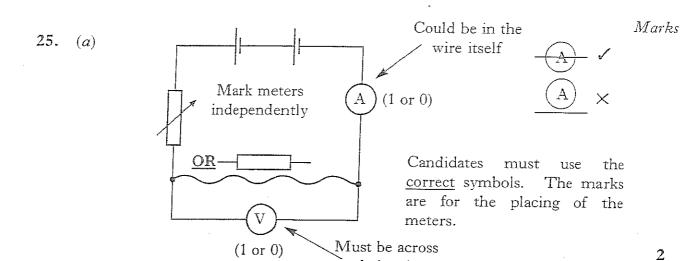
(b) (i) Use variable resistor (to change current in circuit) (1)
