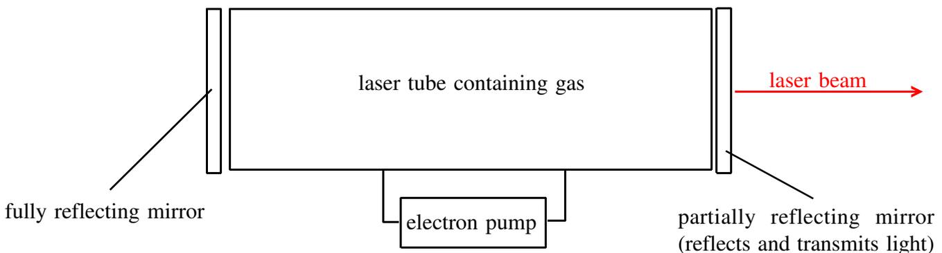
In a **laser**, a gas is contained in a tube with a **fully-reflecting silver mirror** at one end and a **partially-reflecting silver mirror** at the other end.
