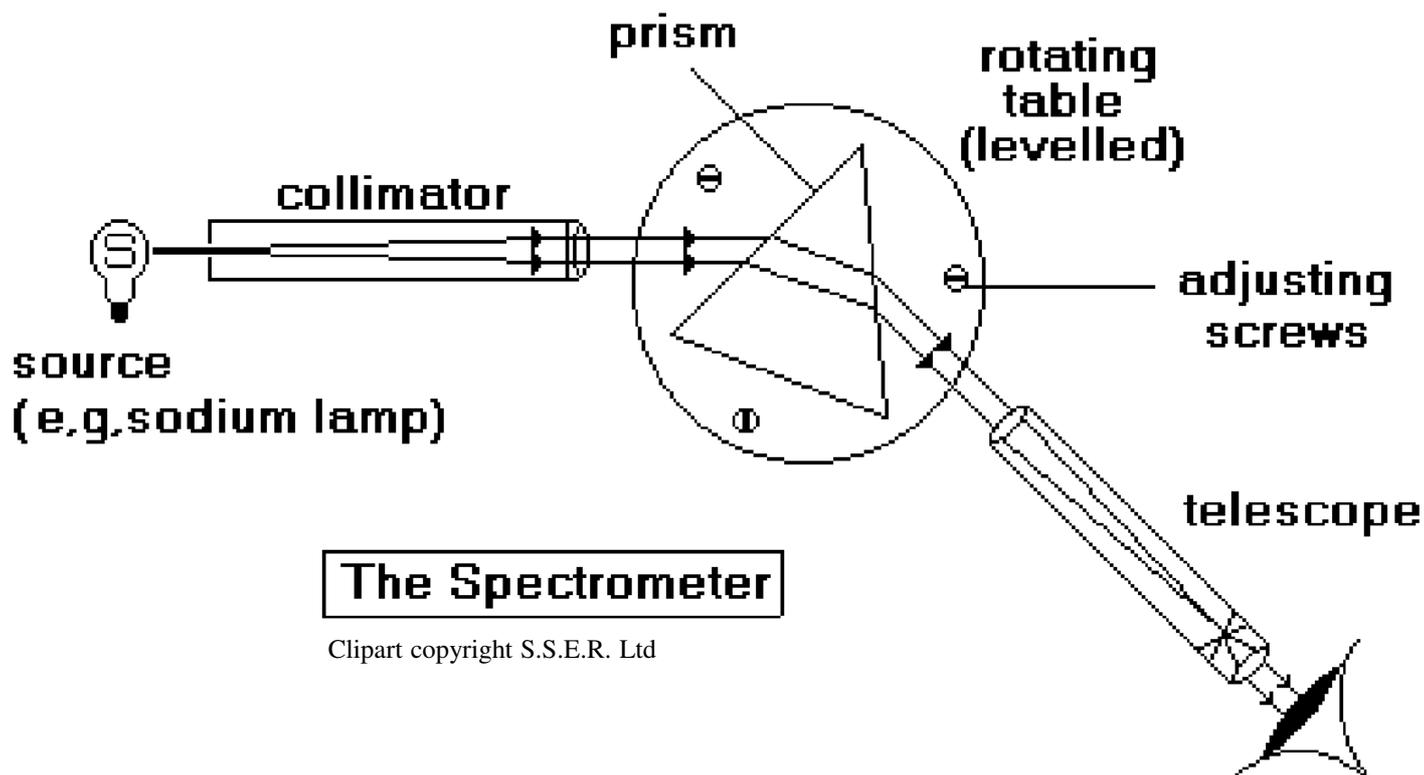
In order to obtain an extremely accurate value for the angle between maxima in a light interference pattern, a device called a **spectrometer** is often used.
