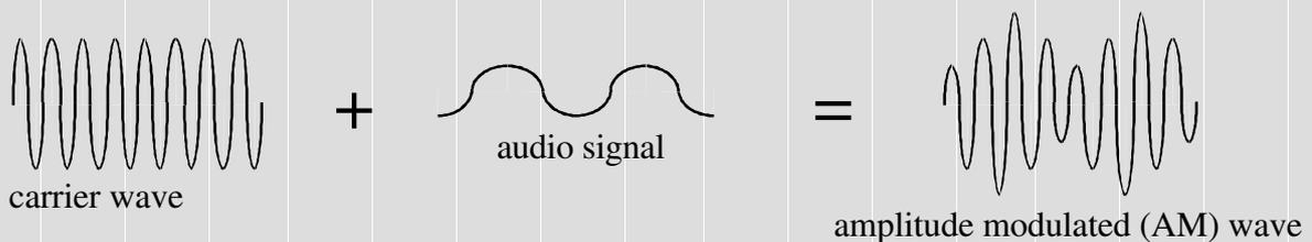
These modulated signals are converted from electrical signals into radio waves at the **transmitter**. The radio waves travel through the air and are then converted back into electrical signals at the **receiver** where the audio signal is extracted from the modulated signal.
