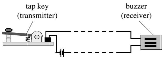
Each letter of the alphabet is encoded as a series of long and short pulses ('dashes' and 'dots') of electricity:
