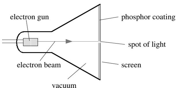
A picture is built up on the TV screen by moving the electron beam across the screen in a series of **lines** (there are 625 lines on a UK TV).
