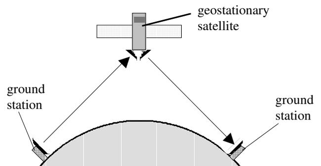
With three geostationary satellites placed in orbit around the equator worldwide communication is permitted with each satellite communicating with ground stations on different continents.
