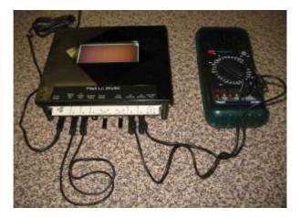
You will have to measure the brightness of the light transmitted through the liquid crystal shutter. You may have to consider the effect of background lighting.
