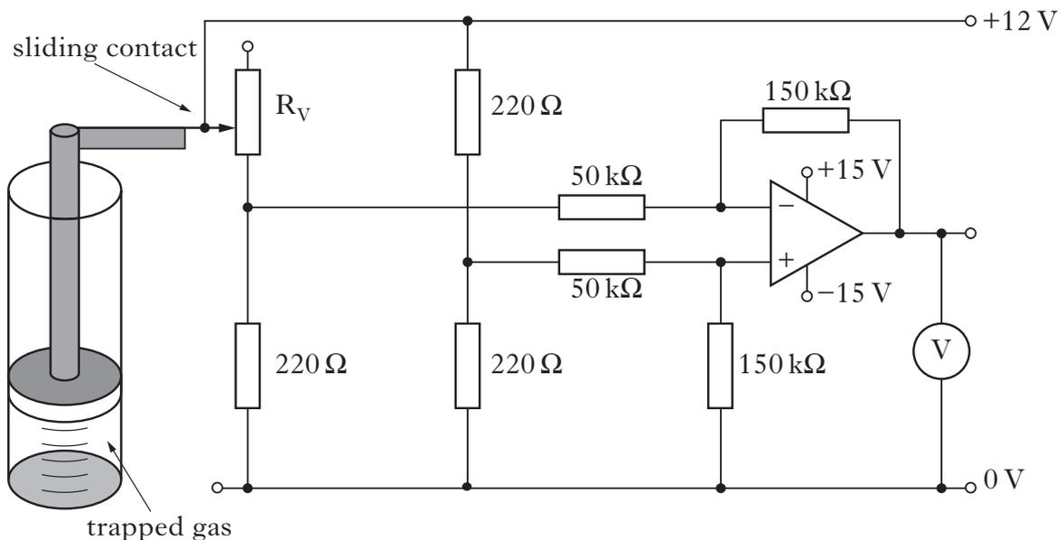
The resistance of  $R_V$  decreases as the depth of the mini-submarine increases.
