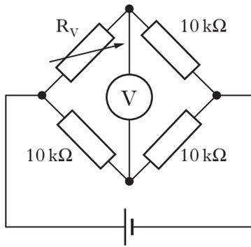
The reading on the voltmeter is zero.
