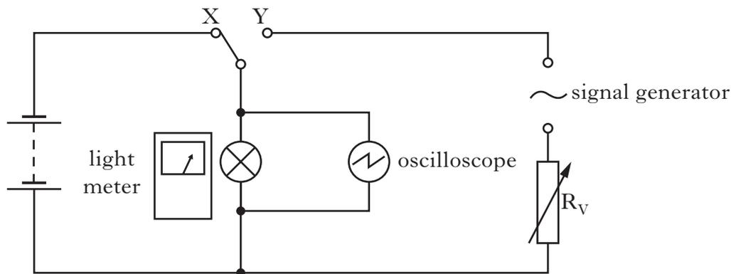
The switch is connected to X and the voltage across the lamp is 2.30 V. The reading on the light meter is recorded.
