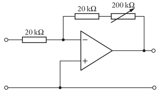
In this circuit, adjustment of the resistance of the variable resistor from zero to  $200\text{ k}\Omega$  allows the voltage gain to be altered over the range
