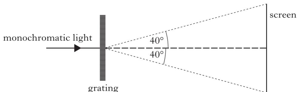
The wavelength of the light is 420 nm and the separation of the slits on the grating is  $3.27 \times 10^{-6}$  m.
