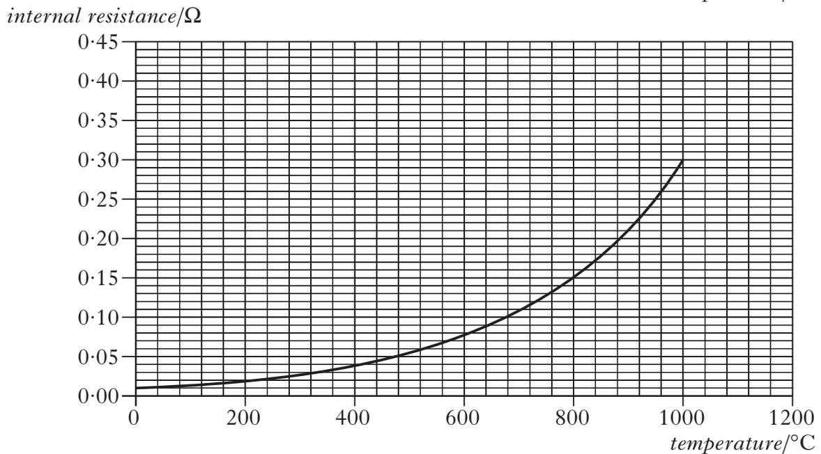
Is this thermocouple suitable as a source of e.m.f. for the gas valve to be open at a temperature of  $800 \text{ }^\circ\text{C}$ ?
