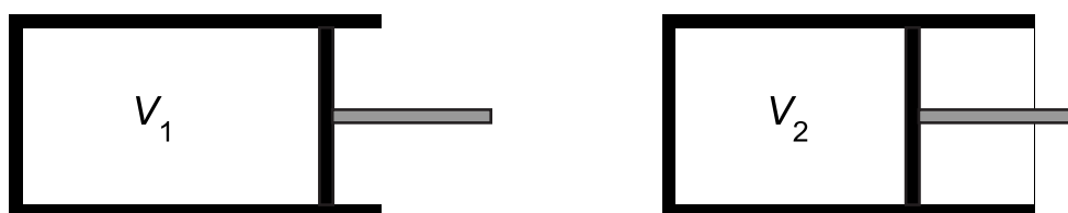
Figure 6.2: A fixed mass of gas at constant temperature being reduced in volume
