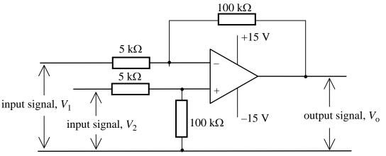
The op-amp has two inputs,  $V_1$  and  $V_2$ . The voltage applied to  $V_1$  is 0.4 V and the voltage applied to  $V_2$  is 0.5 V. Calculate the output from this op-amp.
