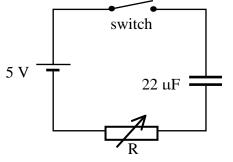
The switch is closed so that the capacitor charges through resistor R.
