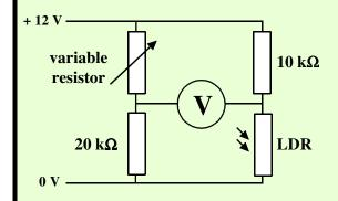
In this Wheatstone bridge circuit, the variable resistor is adjusted until the bridge is balanced
