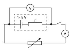
(a) Describe how the student would use this apparatus, and analyse the data obtained, to determine the value for the internal resistance of the cell.
