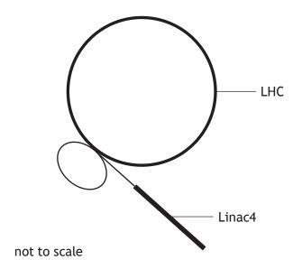
Linac4 accelerates hydrogen ions before they enter the main LHC.
