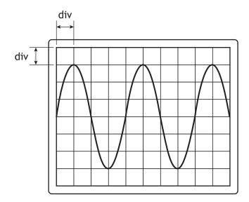
The Y-gain setting on the oscilloscope is 5.0 V/div.
