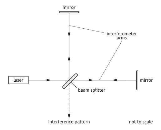
(i) Explain, in terms of waves, how a minimum is formed in the interference pattern.
