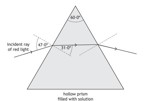
(i) Calculate the refractive index of this solution. (a) Space for working and answer
