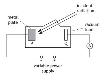
The student notices that when white light is incident on metal plate P, the reading on the ammeter is 0 A. However, when ultraviolet radiation is incident on plate P, the reading on the ammeter is greater than 0 A.
