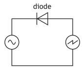
Current can only flow in one direction through a diode.
