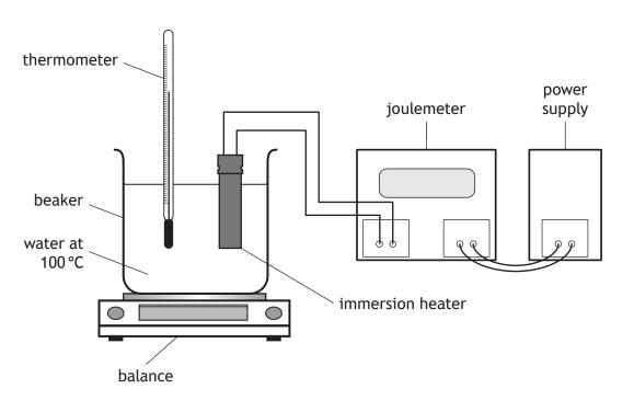
Describe how this apparatus would be used to determine a value for the specific latent heat of vaporisation of water.
