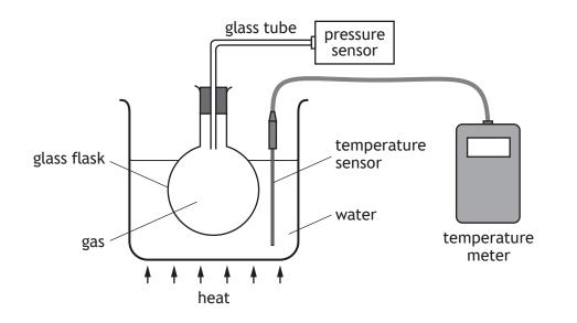
(a) The student heats the water and records the following readings of pressure and temperature.
