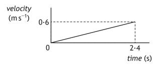
Determine the distance travelled by the trolley in the first  $2 \cdot 4 \, s$  after its release.
