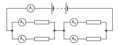
The reading on ammeter  $A_1$  is  $5{\cdot}0\,A.$
