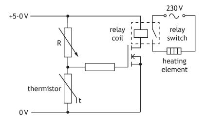
As the temperature of the water increases, the resistance of the thermistor decreases.
