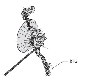
The RTG transforms the heat released by the radioactive decay of plutonium-238 into electrical energy.
