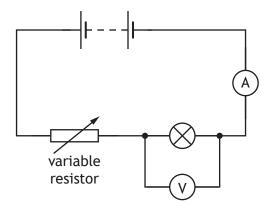
The student uses the circuit to obtain a range of measurements of current in the lamp and voltage across the lamp.
