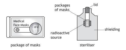
(a) The gamma radiation is produced by a cobalt-60 source.
