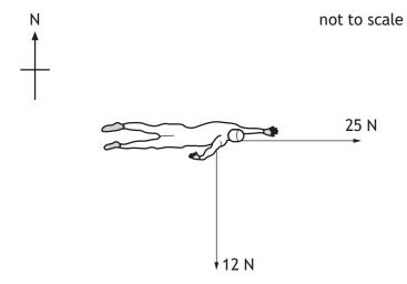
(i) (A) By scale drawing or otherwise, determine the magnitude of the resultant of these forces.
