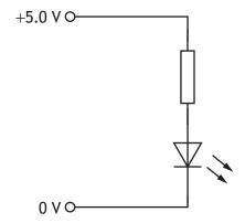
The voltage across the LED is 2.2 V and the current in the LED is 18 mA. Determine the resistance of the resistor in series with the LED. Space for working and answer
