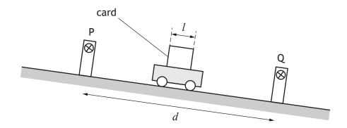
The time taken for the card to pass through light gate P is  $t_1$ .
