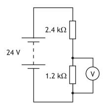
The reading on the voltmeter is
