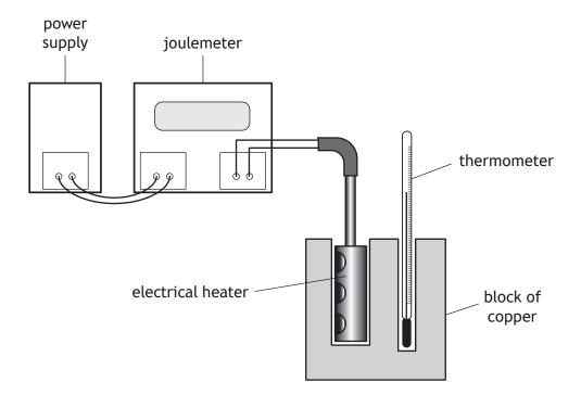
The student switches on the power supply and the electrical heater heats the block of copper.
