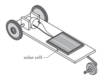
The solar cell produces a voltage of 0.5 V and a current of 0.4 mA.
