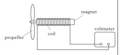
Air blows across the propeller causing the magnet to rotate. A voltage is induced across the coil.
