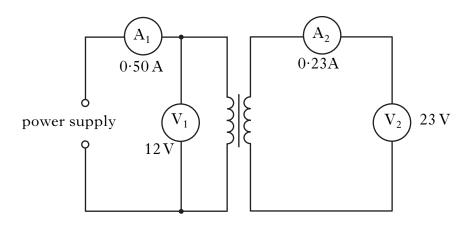
(a) The technician has a choice of an a.c. or a d.c. power supply. Which power supply should be used?Explain your answer.
