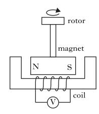
When the rotor is turned the magnet rotates, inducing a voltage in the coil. The induced voltage can be decreased by
