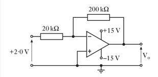
A voltage of +2·0 V is applied to the input. The voltage output,  $\rm V_o,$  is approximately
