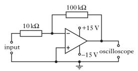
The input has a frequency of 280 Hz and a peak voltage of 0.5 V.
