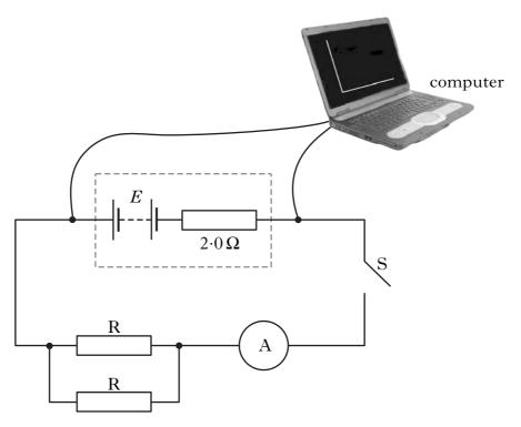
The computer is again connected in order to display a graph of potential difference against time.
