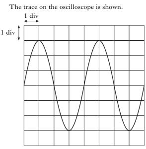
The time-base is set at  $0{\cdot}01\,\text{s/div}$  and the Y-gain is set at  $4{\cdot}0\,\text{V/div}.$
