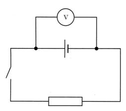
When the switch is open, the student notes that the reading on the voltmeter is  $1.5 \, \mathrm{V}$ . The switch is then closed and the reading falls to  $1.3 \, \mathrm{V}$ .
