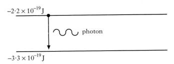
The energy in each pulse of radiation from the laser is 10 J. How many photons are there in each pulse?
