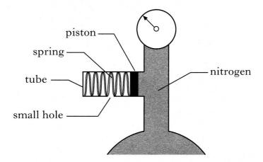
The piston of cross-sectional area  $4.0 \times 10^{-6}$  m<sup>2</sup> is attached to the spring. The piston is free to move along the tube.
