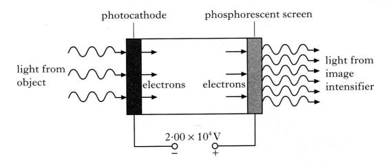
The voltage between the photocathode and the phosphorescent screen is  $2.00 \times 10^4 V$ .
