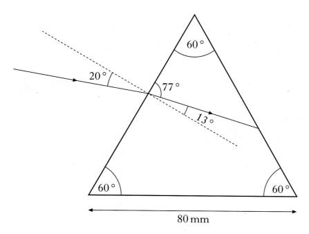
(a) Using information from this diagram, show that the refractive index of the glass for this red light is 1.52.
