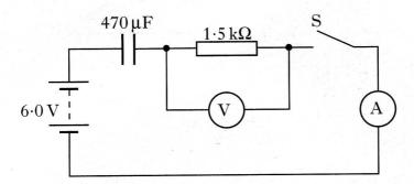
The capacitor is initially uncharged.
