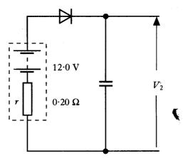
Explain why the voltage  $V_2$  across the capacitor does not decrease from 12.0 V immediately after the car door is opened and the courtesy light comes on.
