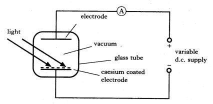
The tube has two electrodes, one of which is coated with caesium. Light of frequency  $6.1 \times 10^{14}$ Hz is shone on to the caesium coated electrode.
