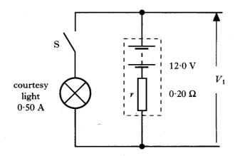
When the car door is opened, the switch S closes and the courtesy light draws a current of  $0.50 \, \text{A}$  from the battery.
