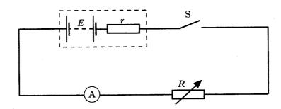
The variable resistor provides known values of resistance R.
