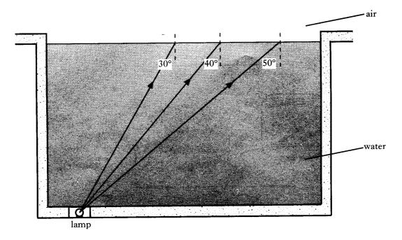
Three rays of light from the same point in the lamp are incident on the water-air boundary with angles of incidence of 30°, 40° and 50°, as shown above.
