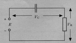
The voltages,  $V_{\rm C}$  and  $V_{\rm R}$ , across the components are recorded at regular time intervals as the capacitor charges up.
