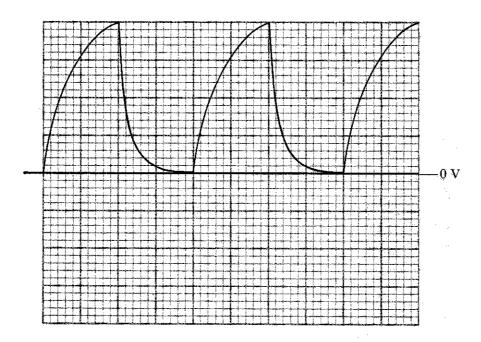
The time base of the oscilloscope is set at 5 ms per centimetre and the Y gain is set at 2 V per centimetre.
