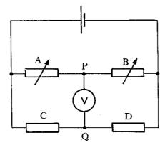
(i) How are the resistances of A, B, C and D related when the bridge is balanced?
