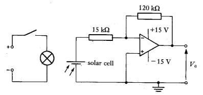
The apparatus is set up near to a window and, with the lamp switched off, there is an output voltage  $V_0$  of -1.75 V.
