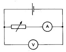
The voltmeter and ammeter readings for a range of settings of the variable resistor are used to produce the graph below.
