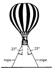
By using a scale diagram, or otherwise, calculate the tension in each rope.
