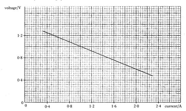
Use the graph to find the values for the e.m.f. and internal resistance of the cell.
