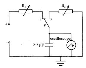
The capacitor is repeatedly charged and discharged by switching S between contacts 1 and 2.
