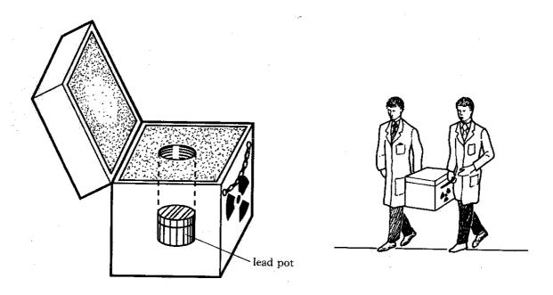
The lead pot provides shielding.
