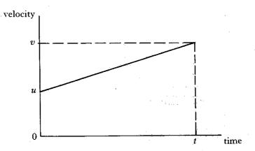
Show that during the time interval t the object moves through a displacement s given by
