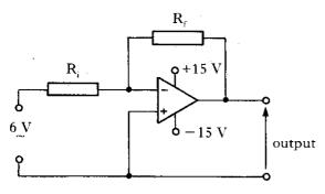
Which values for resistors  $R_i$  and  $R_f$  will produce an approximately square wave output?
