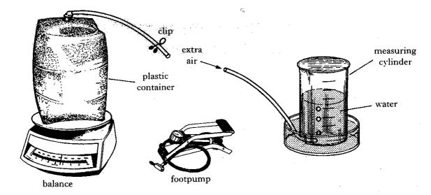
Using the footpump, extra air is pumped into the container. This extra air is released into the measuring cylinder as shown above and its volume measured.
