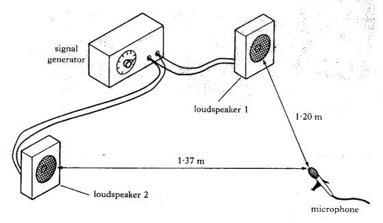
State and explain what happens to the amplitude of the signal picked up by the microphone when loudspeaker 2 is switched on.
