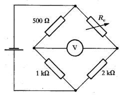
Which of the following would best represent the shape of a graph of the voltmeter reading V against the resistance  $R_r$  as it is varied between 990  $\Omega$  and 1010  $\Omega$ ?
