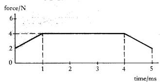
What is the total impulse given to the object by the force in this 5 millisecond time interval?
