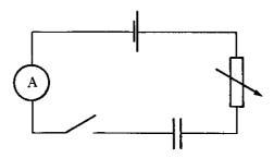
The switch is closed and the capacitor charges up. The variation of current I with time t for this circuit is shown in the following graph.
