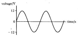
What d.c. supply voltage would produce the same rate of heating from this heater?
