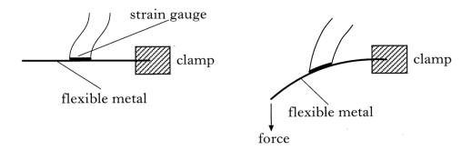
When a force is applied to the end of the piece of metal, it bends.
