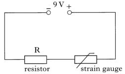
(a) A student is asked to find the resistance of the strain gauge using a voltmeter and an ammeter.
