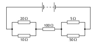
In which resistor is the current smallest?
