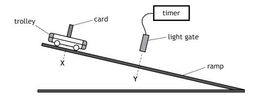
The trolley is released from X and moves down the ramp.
