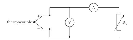
Readings of current and potential difference (p.d.) are recorded for different settings of the variable resistor  $R_{\rm V}.$
