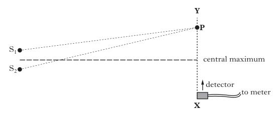
(i) The student moves a microwave detector from X towards Y. The reading on the meter increases and decreases regularly.
