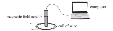
The computer displays values of magnetic field strength. The unit of magnetic field strength is the tesla (T).
