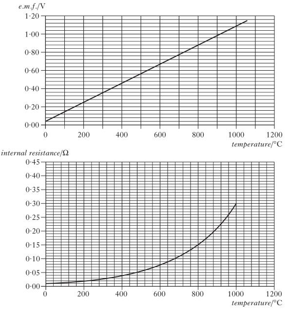
Is this thermocouple suitable as a source of e.m.f. for the gas valve to be open at a temperature of 800 °C?
