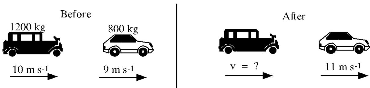
The vehicle at the rear is moving faster than the one in front and they collide. This causes the vehicle in front to be 'nudged' forward with an increased speed. Determine the speed of the rear vehicle immediately after the collision.
