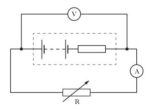
The variable resistor R is adjusted and a series of readings taken from the voltmeter and ammeter.
