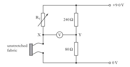
(a) The variable resistor  $R_V$  is adjusted until the bridge is balanced. Show that the resistance of  $R_V$  is now 120  $\Omega$ .
