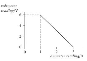
Which row in the table shows the values for the e.m.f. and internal resistance of the battery in the circuit?
