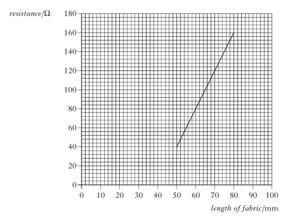
A sample of the fabric of unstretched length 50 mm is connected in a Wheatstone bridge circuit.
