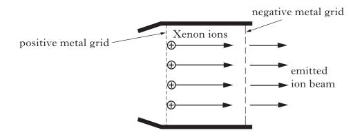
The Xenon ions are accelerated as they pass through an electric field between the charged metal grids. The emitted ion beam causes a force on the spacecraft in the opposite direction.
