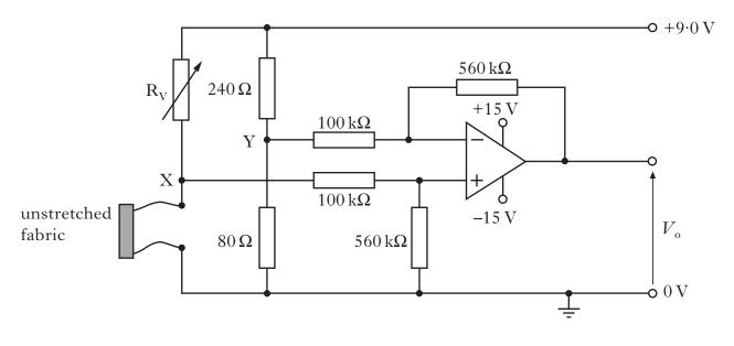
(b) The Wheatstone bridge is now connected to an op-amp circuit as shown.
