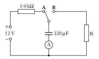
The power supply has an e.m.f. of 12V and negligible internal resistance. The capacitor is initially uncharged.
