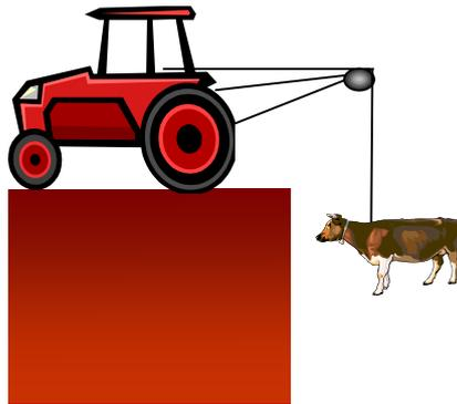
The tractor has a mass of 1500 kg, and the cow has a mass of 500 kg. The tractor's engine can apply a force of 6000 N. Ignore friction between the tractor and the ground.
