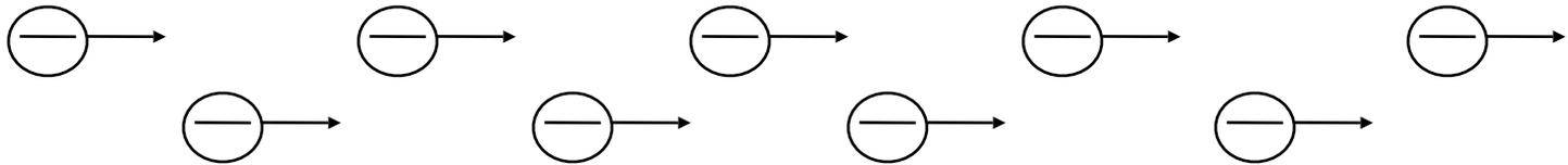
This flow of electric charge is called a current.
