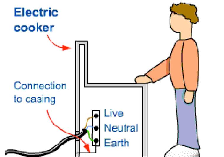
This blows the fuse and switches the appliance off, leaving you safe.
