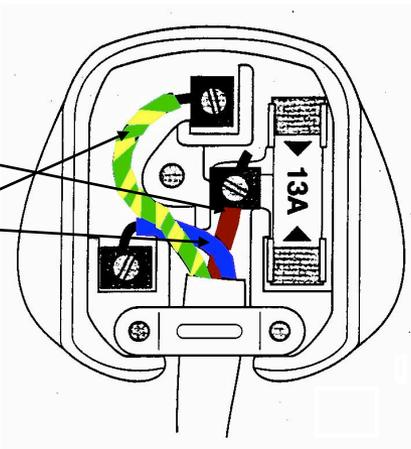
Each of these three wire have different colours of insulation.
