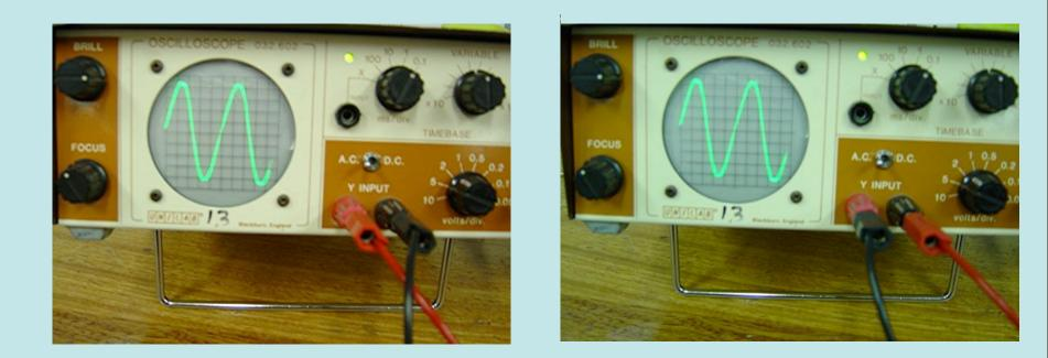
Mains current cycles from positive to negative 50 times per second (50Hz) Signal pattern is the same independent of how the leads are connected
