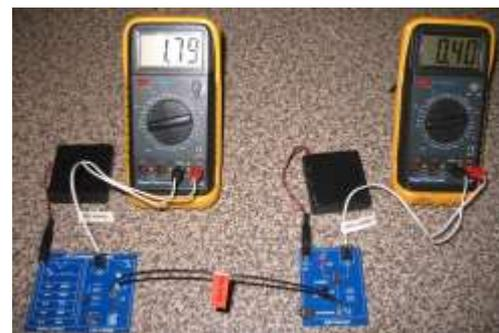
You will have to measure the brightness of the LED. There are light sensors based on photodiodes which can give a voltage which varies directly with the brightness of the light falling on the photodiode. An optical fibre may be used to direct the light from the LED on to the light sensor. It may be necessary to consider the effect of background lighting.
