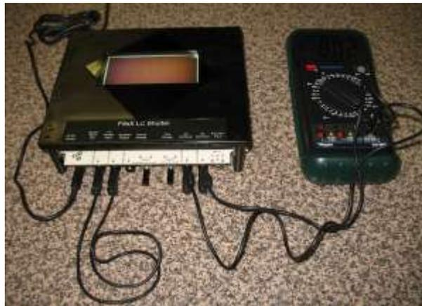
You will have to measure the brightness of the light transmitted through the liquid crystal shutter. You may have to consider the effect of background lighting.
